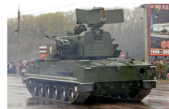
2K22M Tunguska-M; SA-19 tracked self-propelled anti-aircraft weapon armed with surface-to-air gun and missile system.
