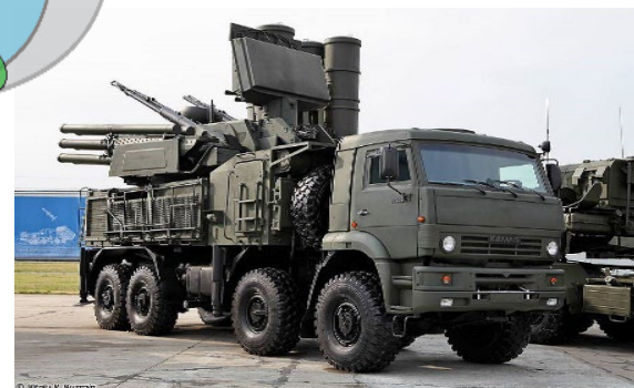
The Pantsir-S1 (SA-22 Greyhound NATO code name) is an air defense missile-gun system designed for the protection of troops and military installations against precision-guided air attack from low and extremely low altitudes.
