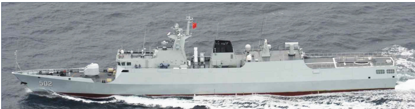
PLAN type 056A corvette Huangshi. The A models denote enhanced littoral warfare capabilities the previous versions did not have, including antisubmarine warfare (ASW) features. Note the hull number 502. The PLAN has since renumbered the early 056A corvettes including the Huangshi. The current hull number for the Huangshi is 655.
