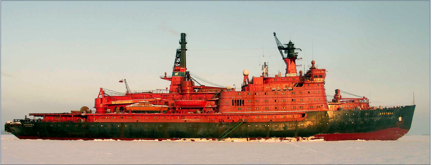
The Russian Nuclear Icebreaker Arktika, the first of its class of nuclear-powered icebreakers.
