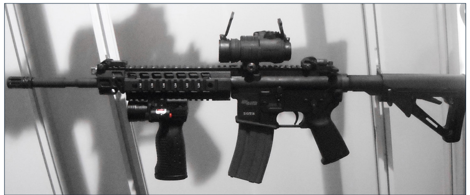
▲ The next generation M4 rifle from Swiss Arms, the Sig Sauer SG 516 is a newborn assault rifle manufactured by the SIGARMS GmbH, Switzerland. The rifle is based on an American-made Colt Defense M4 Carbine but combined with gas piston/op-rod system, based on the SIG 550 series system.
