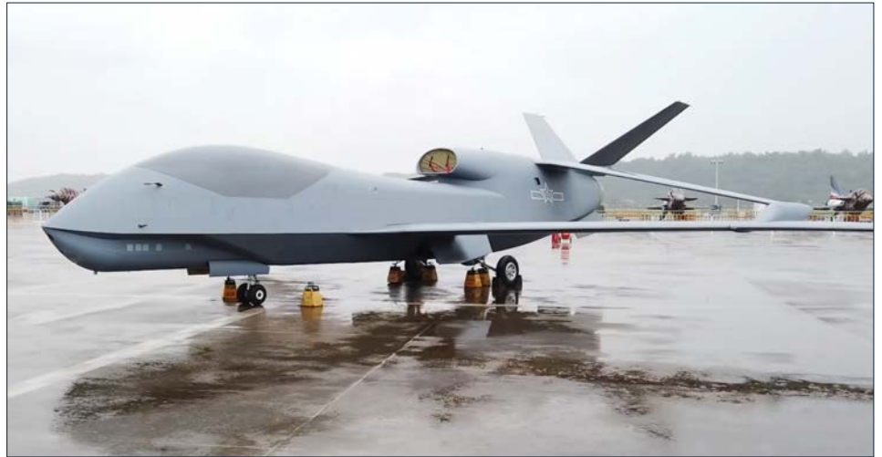
China's WZ-7 ("Soaring Dragon") is a high-altitude, long-endurance drone, shown here on display during the 2022 Zhuhai Airshow.
