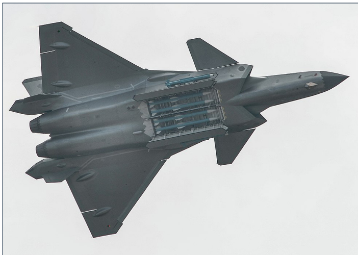
Chengdu J-20 fighter displaying its weapon bays, missiles, and avionics during the 2018 Zhuhai Airshow.
