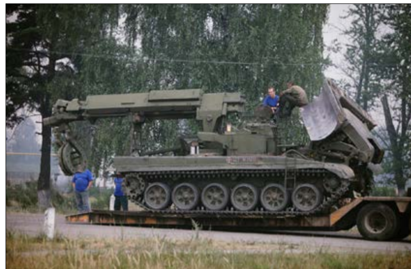
An armored engineering vehicle (IMR) used by the Moscow Military District to fight wildfires in the Moscow Region's Lukhovitsky district. Source: https://commons.wikimedia.org/wiki/File:RIAN_archive_734015_Wildfires_in_Moscow_Region%27s_Lukhovitsky_district.jpg , Attribution: CC BY 3.0
