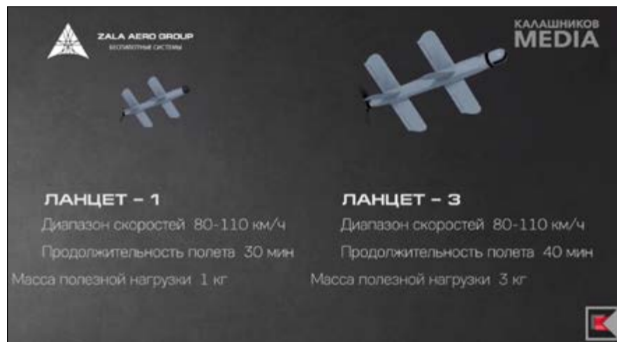
Screen shot from defense manufacturer's promotional film of Lancet loitering munition UAV.
