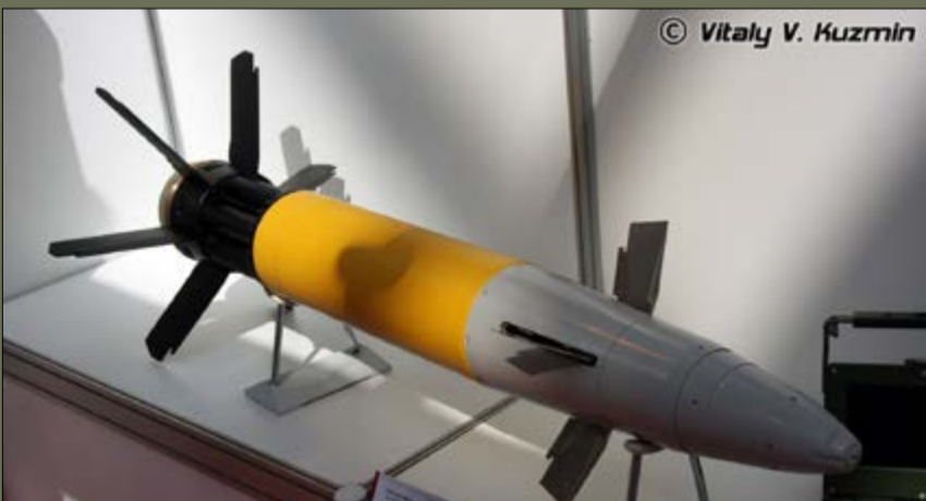
Krasnopol-M2 laser-guided 152mm guided projectile.
