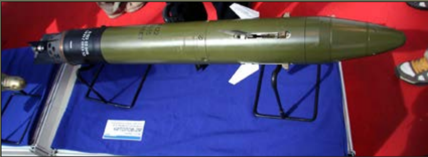
Kitolov-2M laser-guided 122mm guided projectile.
