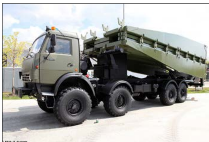
TMM-7 Heavy Mechanical Bridge.
