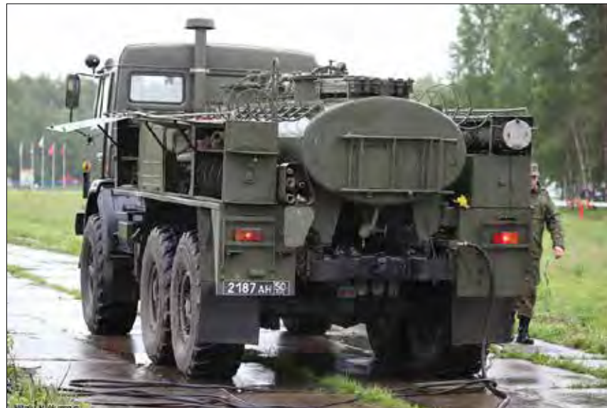
ARS-14KM decontamination and degassing station.
