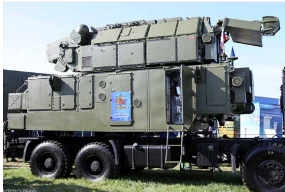
9A331MK-1 autonomous combat module from Tor-M2KM system on TATA chassis. Source: Vitaly V. Kuzmin via Wikimedia, https://commons.wikimedia.org/wiki/File:MAKS_Airshow_2013_(Ramenskoye_Airport,_Russia)_521-38.jpg , CC BY 4.0
