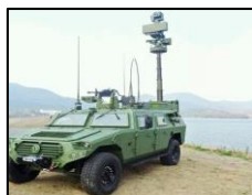
Ground Surveillance Radar can detect personnel at approximately 20km and vehicles up to 40km.
