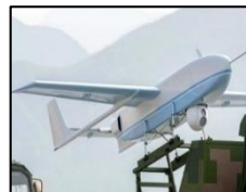
CH-91, also known as BZK-008, is a fixed-wing UAV with inverted v-tail and skids as landing gear. ~20km range.
