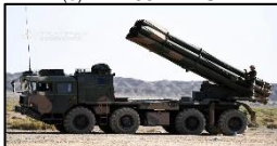
Typically located in the Reserve Zone; has 12 launch tubes for 300 mm artillery rockets with ~130km range.
